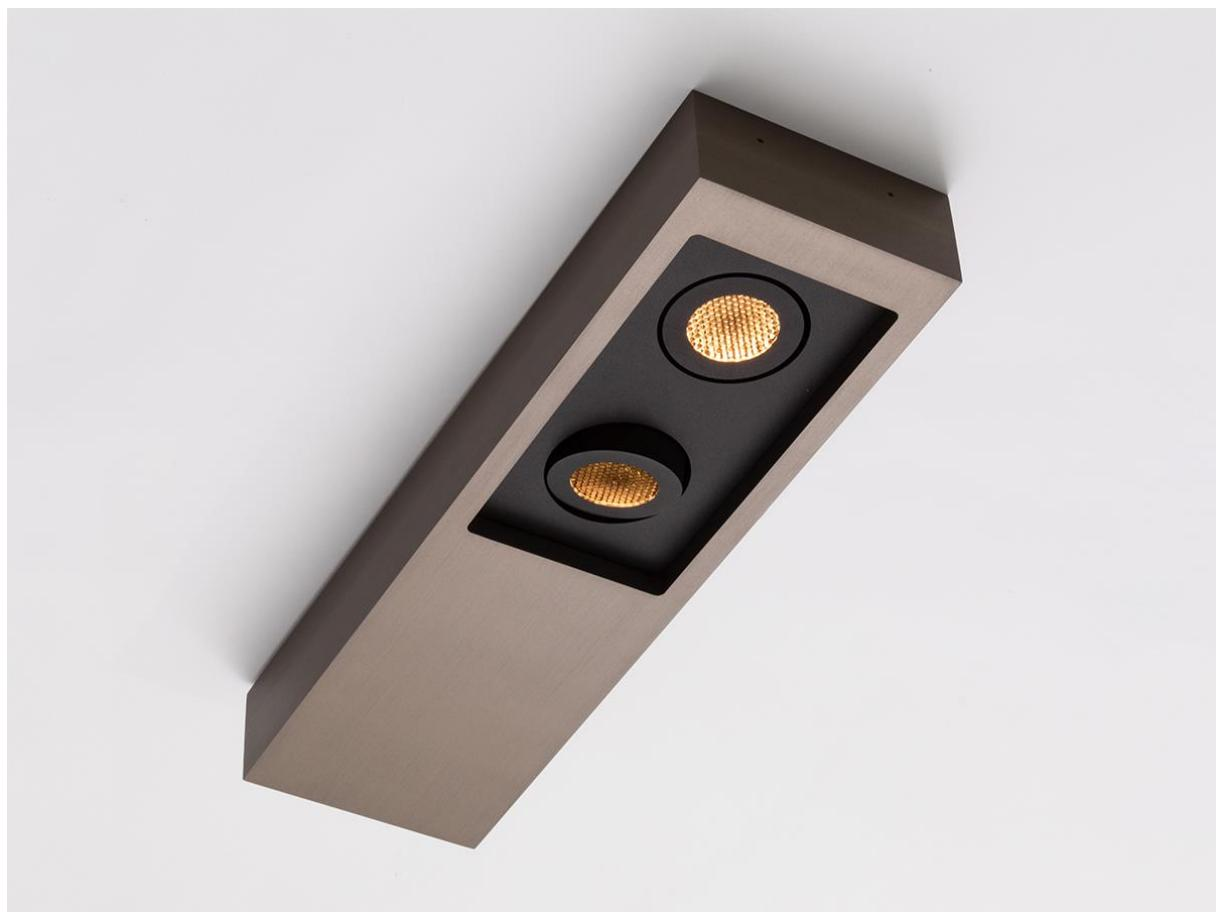
**DESCRIPTION:** Ceiling lamp. Aluminum structure. Finish in medal bronze or satin white. The light fixture has two configurable spotlights. Warm white 2700K LED sources, 24W, 2000Lumens. Each spotlight is adjustable downwards at 0° or 15°. During setting, each spot can rotate at 360° along its axis. Converter 500mA non-integrated, to be placed in a distant box. Weight: 5kg – 11.1lbs Size: 48x14x6cm – 18.9x5.5x2.3in Compliance: CE Class III Origin: France
